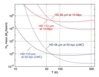
**Figure 4.** Detectable molecular mass in HD as a function of distance and gas temperature, for a flux limit of  $5 \times 10^{-20}$  W m<sup>-2</sup> (SAFARI R = 300).
