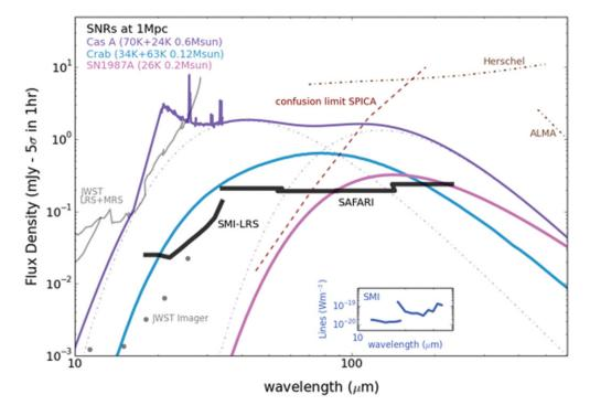
**Figure 8.** Sensitivity comparison for *SPICA* SAFARI and SMI (solid black lines) compared to *Herschel*, ALMA, and *JWST* in dot-dashed grey. The inset shows the  $5-\sigma$ , 1 h levels, line sensitivities for *SPICA* SMI MRS and HRS spectrometers. The confusion limit is shown as a dashed line.
