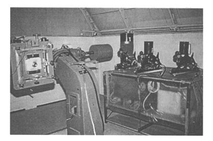
Figure 1. ASAS-3 in the 10" astrograph dome. From the left: 10" astrograph, F = 750 mm telescope, 2 wide-field instruments with 200/2.8 telephoto lenses.
