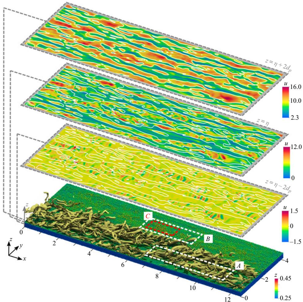
Figure 4. Isometric view of the particle bed from S3 with three horizontal planes showing contours of streamwise velocity. The middle plane is located at the particle bed interface and denoted by  $\eta = z_{\phi=0.1}$ . The other two planes are shifted by two particle diameters above and below the particle bed interface. Below the interface, only KH rollers are present, while above the interface, we only observe longitudinal streaks and do not detect the imprints of the KH rollers.
