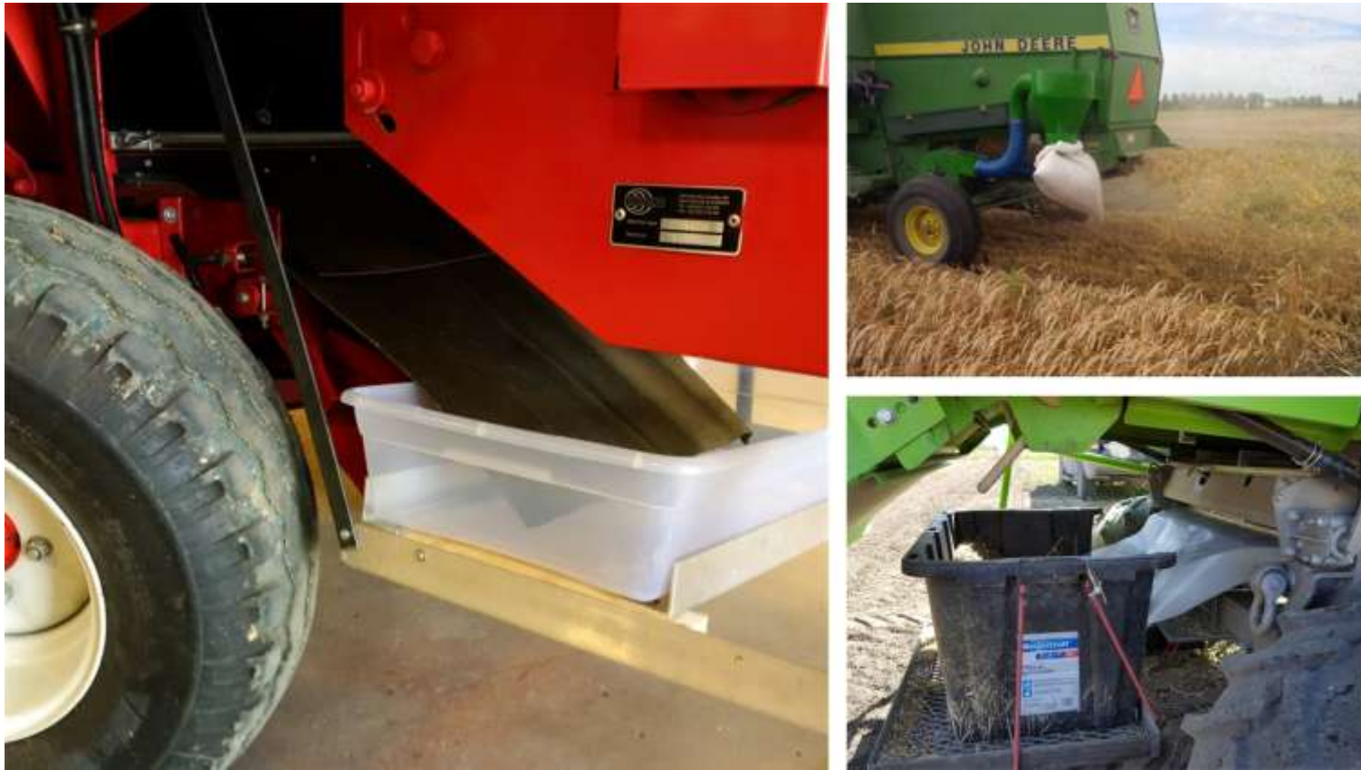
Figure 1. Examples of chaff collection systems used on different plot combines in the study conducted from 2016-2018 to investigate crop rotation maturity, harvest management and harvest weed seed control effects on wild oat populations. Each combine has unique chaff and straw spreading setups and so each chaff collection system was unique to individual locations. These are three examples of systems used in this study.
