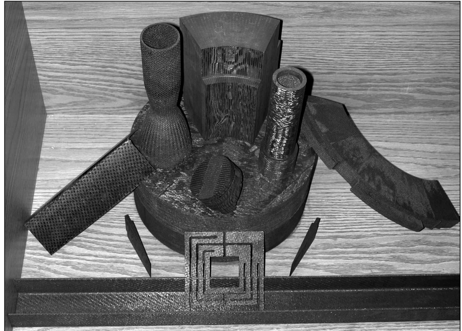
Figure 1. Components fabricated by the in situ rapid densification process include brakes, nozzles, pistons, hypersonic leading edges, heating elements, and structural components.
