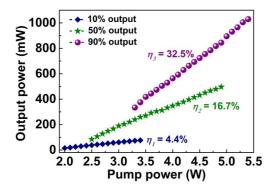
Figure 2. The average output power of TDFLs versus pump power with laser output ratios of 10%, 50% and 90%, respectively.
