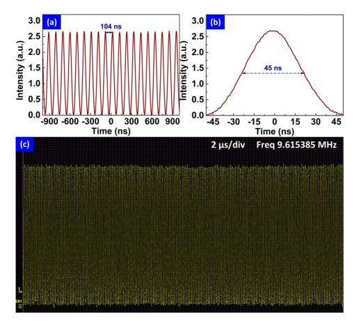
Figure 4. The output pulse trains of IBML TDFL with 90% output ratio: (a) 200 ns/div, (b) 10 ns/div and (c) 2 µs/div.
