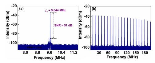
Figure 5. (a) RF spectrum of IBML TDFL with 90% output ratio and (b) broadband RF spectrum.
