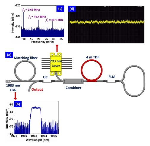
Figure 1. (a) Experimental setup of IBML TDFL with a simple linear cavity, (b) optical reflection spectrum of the 1983 nm FBG, (c) RF spectrum of 793 nm laser and (d) oscilloscope trace of 793 nm laser.
