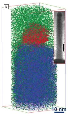
from the silane, which then migrates to the bottom of the drop where it deposits in layers. Significantly more aluminum is thus embedded in the silicon wire than was to be expected theoretically.
