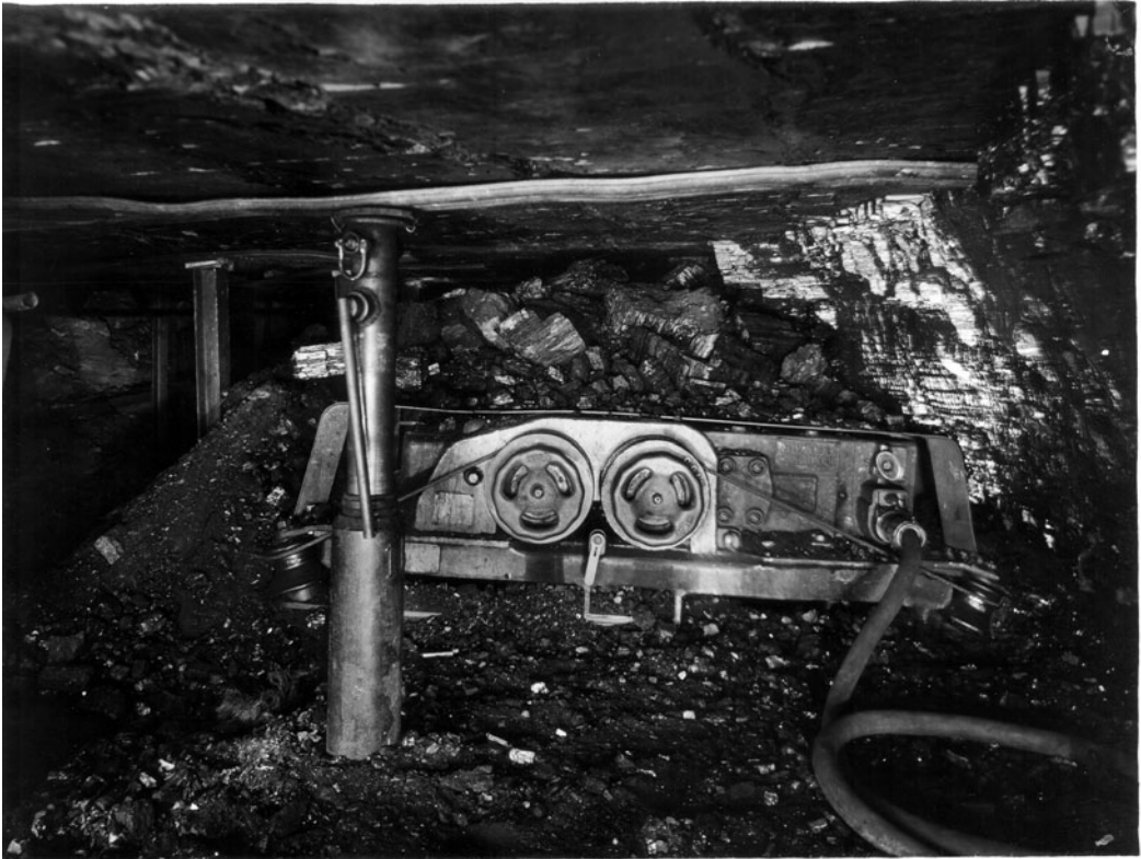
Figure 5. Huwood loader in deep hard seam. (Photograph courtesy of Peasely Colliery Museum).
