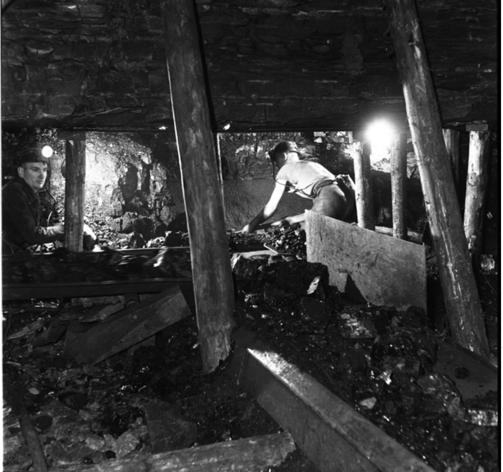
Figure 2. Miners handloading coal onto conveyor. (Photograph courtesy of the National Coal Mining Museum for England).
