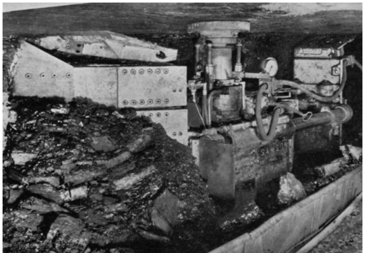
Figure 3. Arcwall Cutter on top of coal in roadway drivage. (Photograph courtesy of Peaseley Colliery Museum).
