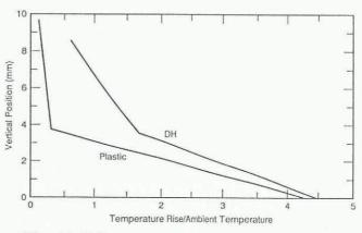
Fig. 12. Relative temperature rise versus vertical position for both skis.
