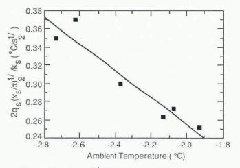
Fig. 4.  $2q_s(\kappa_s/\pi)^{\frac{1}{2}}/k_s$  versus ambient temperature. Other than ambient temperature, the conditions were similar during the various runs.
