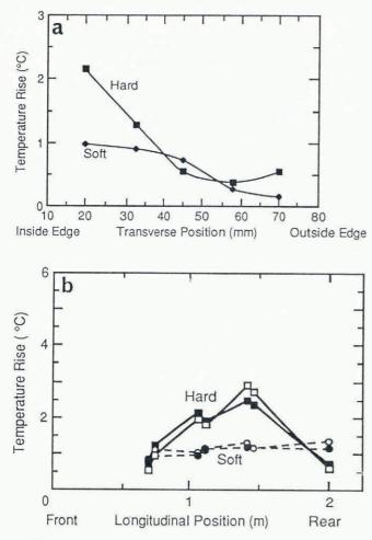
Fig. 9. Basal temperature rise versus position in DH ski runs on days with hard and soft snows. (a) Transverse position, two runs. (b) Longitudinal position, four runs.
