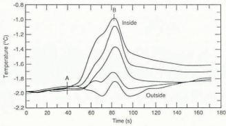
Fig. 8. Basal temperatures from inside to outside of DH skis.  $T_0 = -2^{\circ}C$ ;  $v_{max} \approx 9 \text{ m s}^{-1}$ ; parallel run down gentle slope with load of N/2 on soft, fresh snow.
