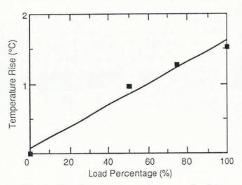
Fig. 6. Basal temperature rise versus load in plastic ski. The 0,0 data point is assumed.
