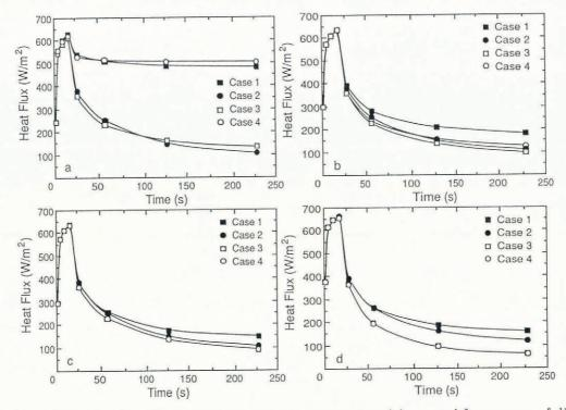
Fig. 13. Computed heat flux versus time for four transverse positions and four cases of different materials as described in the text.  $T_0 = -5 \,^{\circ}C$ ;  $v = 18 \, m \, s^{-1}$ ; load N/2. (a) 3 mm from edge; (b) 100 mm from edge; (c) 25 mm from edge; (d) on center line, 37 mm from edge.
