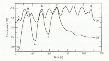
Fig. 5. Basal temperature on right side of plastic ski. (a) Constant-speed ride up Poma lift while cycling the weight on the ski between N and N/2 with a period of 20 s;  $T_0 = -1.8 \,^{\circ}\text{C}$ ;  $v_{max} \approx 2 \, m \, s^{-1}$ ; hard-packed snow. (b) Three periods of start and stop during a parallel run on a gentle slope;  $T_0 = -2.9 \,^{\circ}\text{C}$ ;  $v_{max} \approx 6 \, m \, s^{-1}$ ; load of N on hard-packed snow.
