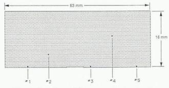
Fig. 1. Locations of thermocouples in the plastic ski in a cross-section under the skier's foot.
