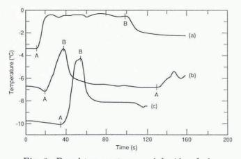
Fig. 2. Basal temperature on left side of plastic ski during parallel runs down gentle slopes. (a)  $T_0 = -3.5 \,^{\circ}C$ ;  $v_{max} \approx 8 \, m \, s^{-1}$ ; load N/2 on soft, fresh snow. (b)  $T_0 = -6.7 \,^{\circ}C$ ;  $v_{max} \approx 6 \, m \, s^{-1}$ ; load N on hard-packed snow. (c)  $T_0 = -9.7 \,^{\circ}C$ ;  $v_{max} \approx 6 \, m \, s^{-1}$ ; load N on hardpacked snow. A indicates starting of motion and B indicates stopping in all graphs.
