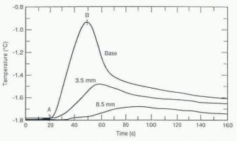
Fig. 11. Vertical temperature profile of DH ski showing basal, 3.5 and 8.5 mm responses.  $T_0 = -1.8^{\circ}$ C;  $v_{max} \approx 9 \, m \, s^{-1}$ ; parallel run down gentle slope with load N/2 on soft, fresh snow.
