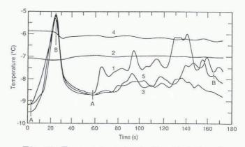
Fig. 10. Temperatures in plastic ski. 1, 3 and 5 are on base in left, middle and right side. 2 is 3.8 mm above and 4 is 9.7 mm above base.  $T_0 = -9.3^{\circ}$ C;  $v_{max} \approx 6 \text{ m s}^{-1}$ ; parallel run down gentle slope with load N on hard-packed snow then up Poma lift at  $\approx 2 \text{ m s}^{-1}$ .
