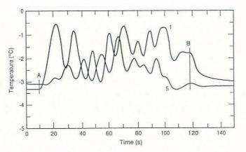
Fig. 7. Basal temperatures on left and right sides of plastic ski during many turns. 1 is the inside and 5 is the outside of the ski.  $T_0 =$  $-3.2^{\circ}$ C;  $v_{max} \approx 6 m s^{-1}$ ; wide, smooth turns with load of N/2 on soft, fresh snow.
