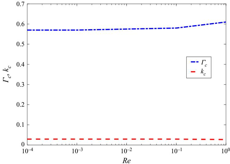
FIGURE 9. The variation of  $\Gamma_c$  and  $k_c$  with  $Re$  at  $a = 0.6$ ,  $b = 1$ ,  $\mu_r = 0.5$ ,  $V_r = 0$ ,  $\Sigma_1 = 1$  and  $\Sigma_2 = 1$ . The figure illustrates the stabilising effect of inertia on the viscous instability. The viscous instability remains the dominant mode of instability for  $Re < 1$ .
