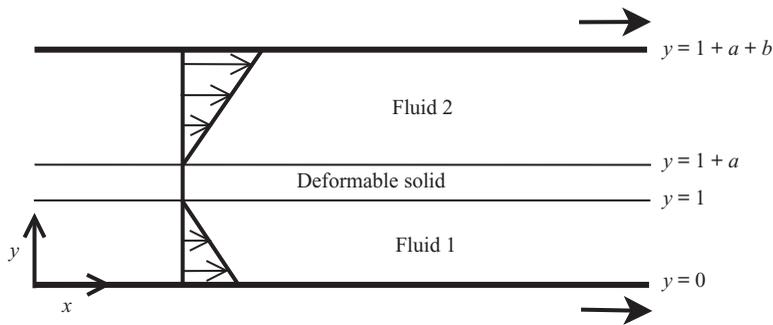
FIGURE 1. Schematic of the flow geometry in dimensionless coordinates. The plates at  $y = 0$  and  $y = 1 + a + b$  are moving with dimensionless speeds 1 and  $V_r$ , respectively. The fluids exert a shear stress at the fluid–DS interface, leading to deformation of the DS and coupling between the base-state fluid motion and perturbations in the DS, which affects the stability of the flows.
