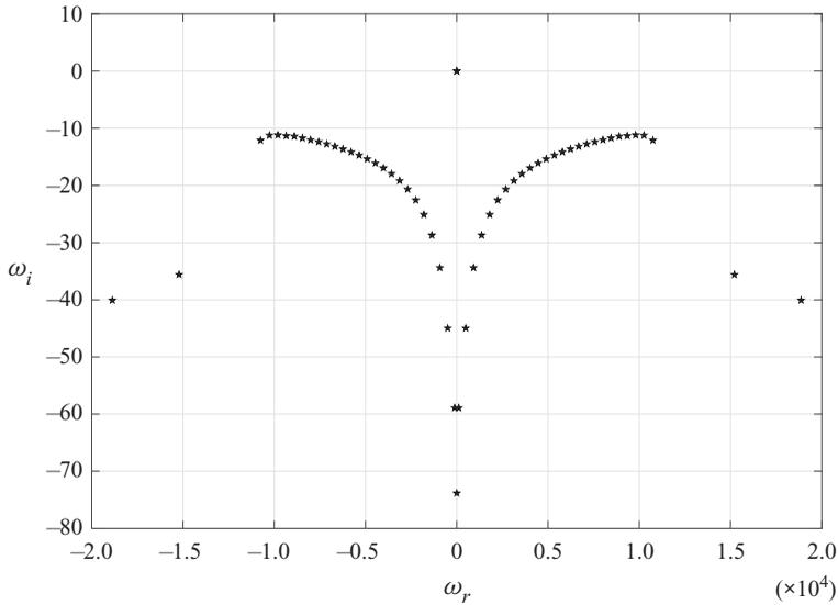
FIGURE 8. The eigenvalue spectrum at  $Re = 0.1$ ,  $a = 0.1$ ,  $b = 1$ ,  $\mu_r = 0.5$ ,  $V_r = 0$ ,  $\Gamma = 0.05$ ,  $k = 0.05$ ,  $\Sigma_1 = 1$  and  $\Sigma_2 = 1$ . The shear waves arising due to the interaction of the fluids and DS are symmetrically distributed about  $\omega_r = 0$  line. The unstable viscous mode of instability,  $\omega = 0.013500 + 0.000727i$  is located on the symmetry line of the spectrum.
