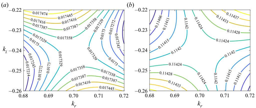
FIGURE 11. The existence of the first-order saddle point,  $k_0 = 0.7010 - 0.24125i$  in the  $k$ -plane corresponding to the cusp point shown in figure 10. The parameters are,  $a = 10^{-4}$ ,  $b = 2$ ,  $\mu_r = 0.1$ ,  $V_r = 0$ ,  $\Gamma = 10^{-3}$ ,  $\Sigma_1 = 1$  and  $\Sigma_2 = 1$ . Panels (a) and (b) show iso-contours for  $\omega_i$  and  $\omega_r$ , respectively. The figure shows the presence of the first-order saddle point in the present model.
