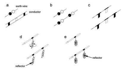
Figure 2. Design of wire markers at 380 kV (a), 220 kV (b) and 110 kV (c) high voltage power lines in Eastern Austria and design of rectangular (d) and circular (e) bird flight diverters used at high- and medium voltage power lines in Western Hungary, attached to the earth wire and conductor, respectively.
