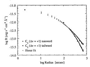
Figure 11. The C<sub>2</sub> profile of comet Halley, measured using an IIDS at the Kitt Peak 2.1-m telescope. The difference between the sunward and tailward profiles is the result of radiation pressure. Figure is from Luu (1988).
