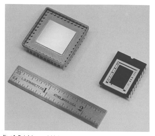
Figure 2. Typical charge coupled devices used for cometary photometry. The larger CCD is a virtual phase TI 4849 with 584 x 390 pixels, and the smaller a TI 850 x 750. The scale ruler is 2.5 inches in length. Figure courtesy of Gerry Luppino, MIT.
