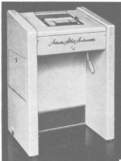
The E.M.40 Clinical Model has facilities for Air and Bone Conduction Tests with pure tones . . . Speech Tests both live and recorded . . . Loudness Balance (Fowler-recruitment) Tests . . . and Malingering Tests. Masking is effected with a "white" noise, which can also be used for the new tests devised by Prof. Langenbeck. Click-less tone interruption is provided. Discrete frequencies—from 64 to 1024 c/s at octave intervals, and from 1024 to 11584 c/s at half-octave intervals—may be selected.
