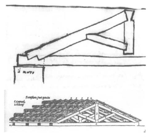
Figure 5. Guidobaldo's sketch (del Monte ca. 1587-1592, 237) and a contemporary representation of a roof with "capriata" (illustration by Palladio, reproduced from Tampone 1996, 71)
