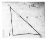
When a descent [caduta] will be of a height of ten, in order to give water to a mill the channel should be 15 [sic!], as the descent ab and the channel ac. But due to the general rule, ac should usually be elevated by ca. 45 degrees, according to the consideration of the quantity of water which one has. (del Monte ca. 1587-1592, 236)
