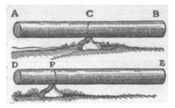
If two places are taken in the length of a cylinder at which the cylinder is to be broken, then the resistances at those two places have to each other the inverse ratio [of areas] of rectangles whose sides are the distances of those two places [from the two ends.]<sup>1</sup>
