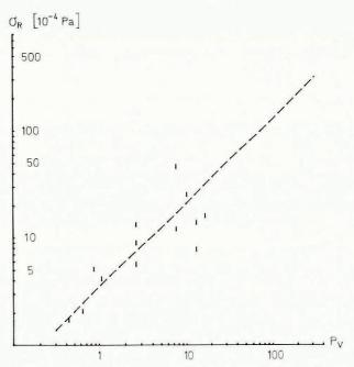
Fig. 9. Strength index or as a function of the mesh parameter Pv.
