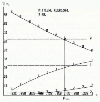
Fig. 4. Example of the determination of  $\bar{n}_3$  by comparing the measured distributions of the  $n_2$  with the corresponding calculated distribution for a given probability p.
