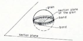
Fig. 2. Sketch of a grain cut by a section plane.
