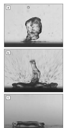
(a) Tornado lift-off of cold water impacting a ceramic heated to 175°C and (b) water jet occurring on the same surface heated to 300°C. (c) Appearance of the droplet after applying the hydrophobic coating to the alumina ceramic. Credit: AIP Advances.
