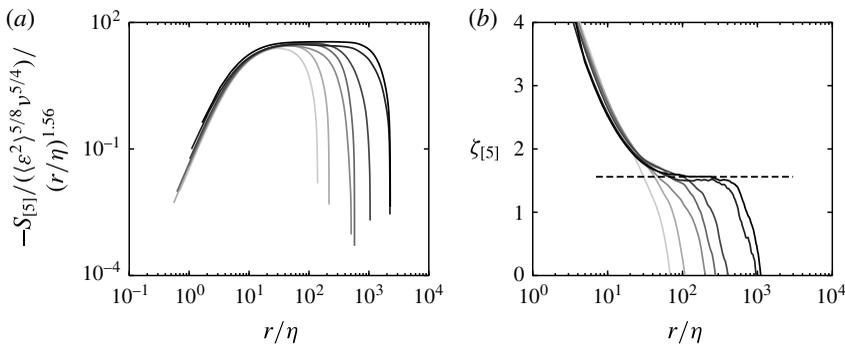
FIGURE 5. Compensated structure function  $S_{[5]}$  in the inertial range for the cases R0–R6 with  $Re_\lambda$  ranging from 88 to 754 (a) and scaling exponent  $\zeta_{[5]}$  (b). Higher Reynolds numbers are indicated by darker shading. The horizontal dashed black line in (b) indicates  $\zeta_{[5]} = 1.56$ .
