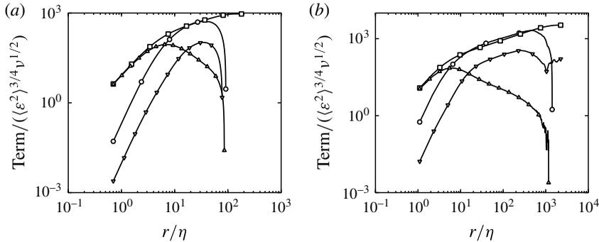
FIGURE 1. Balance of the different terms in (2.4) for the cases  $R0$  ( $Re_\lambda = 88$ ) (a) and  $R5$  ( $Re_\lambda = 529$ ) (b):  $\circ$ , transport term;  $\square$ , dissipative source term;  $\nabla$ , pressure source term;  $\Delta$ , viscous term.
