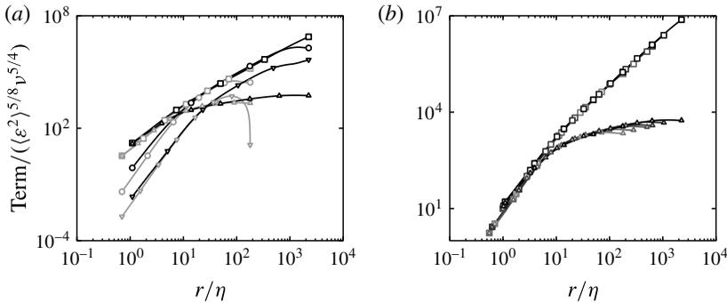
FIGURE 3. (a) Terms of (2.4) numerically integrated over  $r$  for cases  $R0$  (grey) and  $R5$  (black), where  $\circ$  is the transport term,  $\square$  is the dissipative source term,  $\nabla$  is the pressure source term and  $\triangle$  is the viscous term. The integrated dissipative source term  $\square$  and integrated viscous terms  $\triangle$  for all cases  $R0$ – $R5$  (from light grey to black) are shown in (b).
