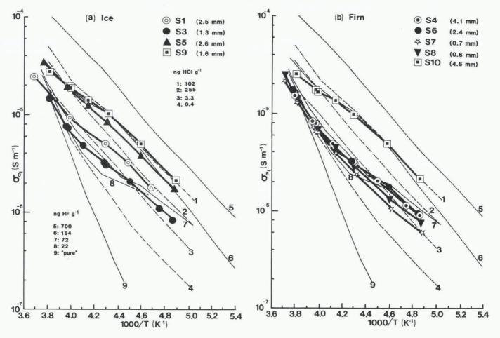
Fig. 5. Solid-phase high-frequency conductivities ( $\sigma_{\infty}$ ) of HCl-doped ice (from Gross and others, 1980, nos. 1-4) and of HF-doped ice (from Camplin and others, 1978, nos. 5-9) compared with  $\sigma_{\infty}$  (heavy lines) of (a) four ice samples and (b) five firn samples from the Antarctic Peninsula. Approximate grain-size of each sample is given in brackets.
