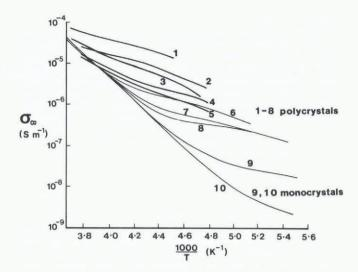
dependence of the high-frequency Fig. 6. Temperature conductivity  $\sigma_{\infty}$  (at 100 kHz unless stated otherwise):
