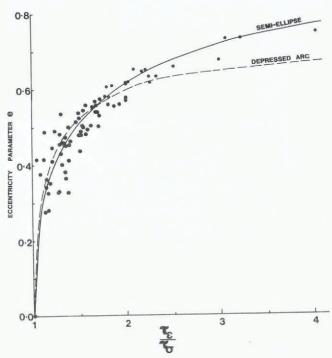
Fig. 1. Eccentricity parameter e as a function of the ratio of relaxation times from complex conductivity ( $\tau_{\sigma}$ ) and complex permittivity ( $\tau_{\epsilon}$ ) dispersions. The dashed and solid lines have been derived from the theory of depressed arcs (Equation (4)) and of semi-elliptical dispersions (Equation (5)), respectively. The dots are experimental values.
