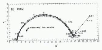
Fig. 2. Dielectric response of (a) sample S3 and (b) sample S8. Frequencies in kHz.
