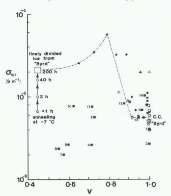
Fig. 7. Ice-volume fraction (v) dependence solid-phase high-frequency conductivity ( $\sigma_{\infty}$ ) at -45°C for samples described in the sources listed in Table III.
