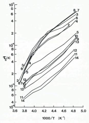
Fig. 4. Temperature dependence of relaxation times  $(\tau_{\epsilon})$  for 14 firn and ice samples from the Antarctic Peninsula.
