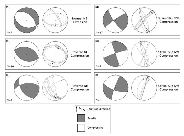
Fig. 3. Fracture results and interpreted stress fields from Kirchleus Quarry showing the main deformation phases affecting the Malm at the outcrop (Köhler et al., 2022).
