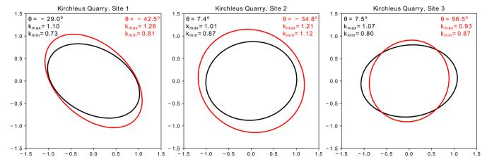
Fig. 7. Permeability ellipses from the homogenization process and tensor calculation. Black permeability ellipse is calculated using a constant permeability for all fractures. Red permeability ellipse is calculated using varying permeabilities based on fracture orientation. Site 1 shows tilting of the ellipse towards the main Kulmbach Fault. Sites 2 and 3 show lessening impact of the fault to the ellipse orientation and magnitude.
