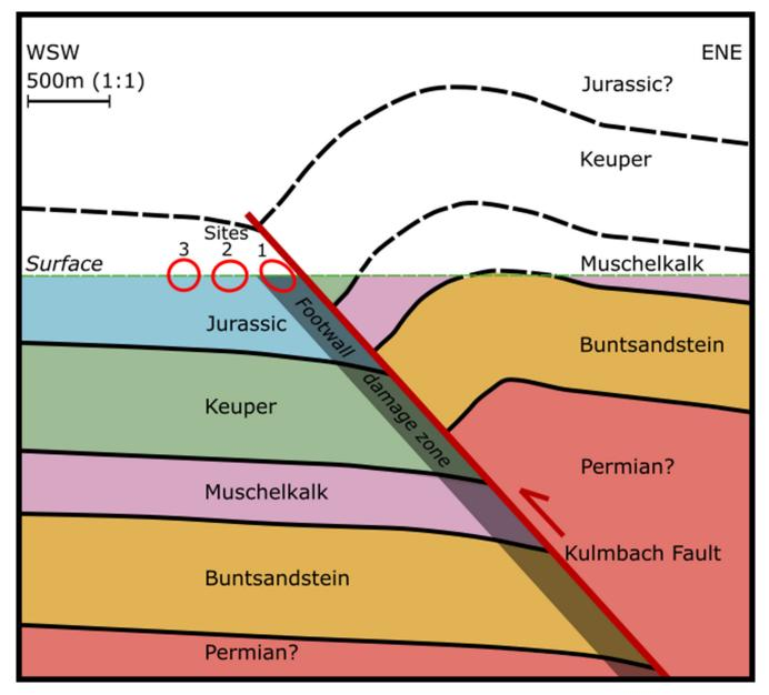
Fig. 9. Conceptual model showing a cross-section through the Kulmbach Fault and how the homogenized permeability of the fracture networks is affected by the fault within the fault damage zone.
