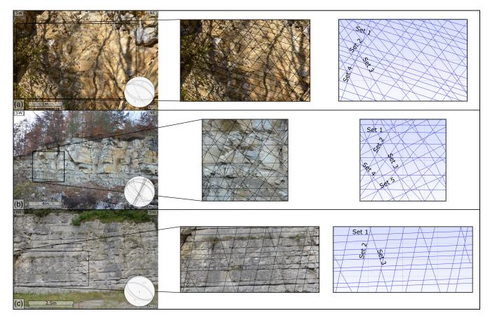
Fig. 4. Fractured cliff sections and digitized interpreted fracture traces from Kirchleus Quarry. Sets identified in fracture traces correspond to the sets presented in Table 1.
