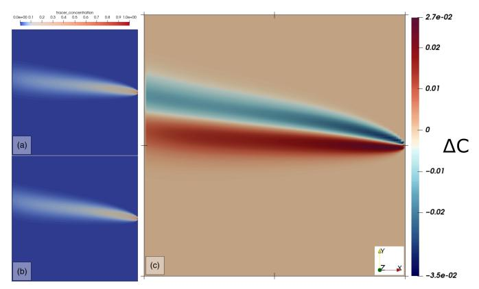
**Fig. 8.** (a, b) Tracer transport through a 5 m × 5 m block using (a) constant permeability for all fractures and (b) variable permeability controlled by fracture orientation and defined conduit, barrier and conduit–barrier sets. (c) Difference in tracer concentration between the two scenarios. Simulations were performed using the PorousFlow module (Permann *et al.* 2020; Wilkins *et al.* 2021) within MOOSE.
