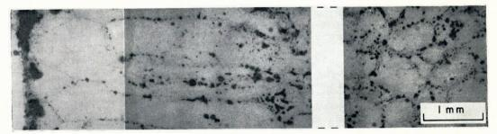
Fig. 9. Reaction patterns obtained from bulk ice frozen from a low concentration NaCl solution.
