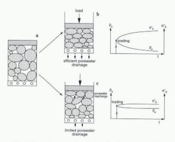
Fig. I. Geostatic compaction of a clastic sediment (a) with pore-water drainage (b) and with limited pore-water drainage and pore-water recharge (c) (modified after Boulton and Dobbie, 1993).  $p_w$  is pore-water pressure,  $\sigma'_z$  is effective stress. (c) illustrates a subglacial system with low hydraulic permeability under a warm-based glacier. Note only slight changes in  $p_w$  and  $\sigma'_z$  after loading in (c).
