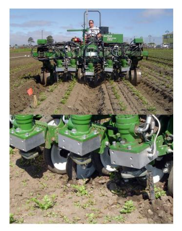
Figure 1. Robocrop intrarow cultivator used on two celery [*Apium graveolens* L. var. dulce (Mill.) DC.] beds at Salinas, CA (top). The bottom photo is a close up of the intrarow cultivation. (Color for this figure is available in the online version of this article.)
