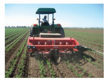
Figure 3. Steketee IC, equipped with reciprocating knives operating in a fennel (*Foeniculum vulgare* Mill.) planting near Castroville, CA. (Color for this figure is available in the online version of this article.)
