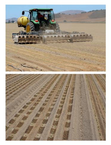
Figure 4. Lettuce thinning at Salinas, CA with the BlueRiver Lettuce Bot (top) and a close-up of the newly thinned lettuce showing the sprayed zones where lettuce will be removed and unsprayed zones where "saved" lettuce plants will be grown to maturity (bottom). (Color for this figure is available in the online version of this article.)
