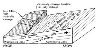
TEXT-FIG. 1.—Minor structures in the small quarry at the top of the cliff just north of the main California Quarry, Boscastle. The quarry face trends N. 60° E.–S. 60° W. and faces N.N.W. An early slaty cleavage and associated linear structures are deformed by later minor folds, overturned to the north, with strain-slip cleavage. Solid arrow shows the facing direction of bedding on slaty cleavage.
