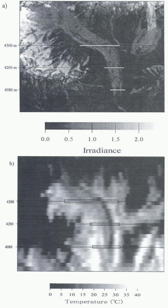
Fig. 4. Distribution of a) high radiation intensity in TM 2 and b) surface temperature from TM Band 6 of LANDSAT 5 on 8 May 1989 in the debris-covered area of the Lirung Glacier.
