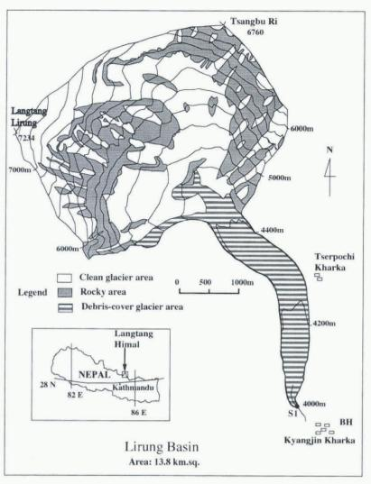
Fig. 1. Topographical map of the Lirung basin in Nepal. S1 shows the location of the hydrological station and BH represents the "Base House" where the meteorological observations were made.
