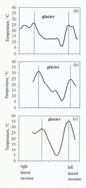
Fig. 5. Transversal temperature profile along the white lines indicated on Fig. 4a of the Lirung Glacier derived from LANDSAT 5 TM Band 6 on 8 May 1989 at a) 4300 m, b) 4200 m and c) 4080 m a.s.l.
