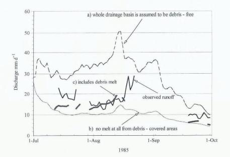
Fig. 6. Comparison of daily observed discharge to simulated runoff in the Lirung drainage basin using the HYCYMODEL, including the melt from the debris zones.
