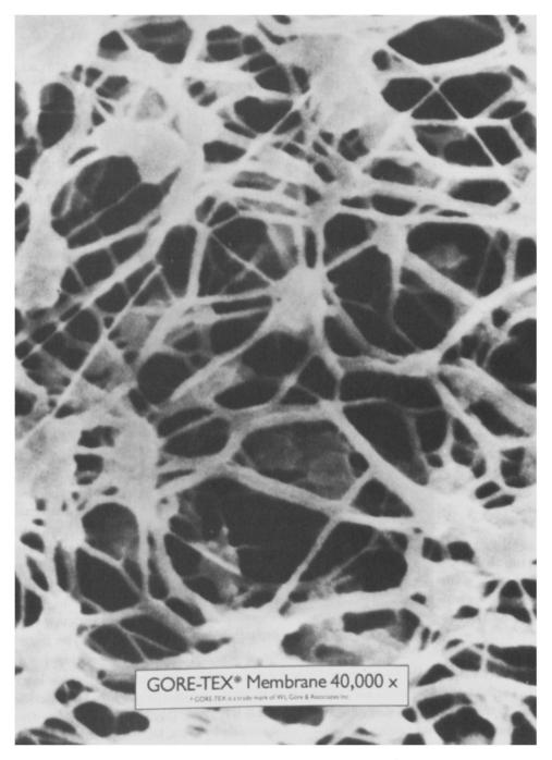
Fig. 1. Scanning electron microscopy photograph for expanded polytetrafluoroethylene membrane × 40000.
