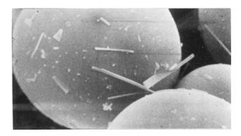
Fig. 3. A  $27\mu$  sphere with surface irregularities that induce a rotational spin (magnification 2600x).
