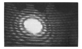
Fig. 2. The far field or Mie scattering pattern in the forward direction for the pair of particles in Figure 1.
