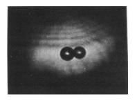
Fig. 1. Near field image of a pair of spheres levitated in an argon laser beam. The spheres are  $20\mu$  and  $25\mu$  in diameter.
