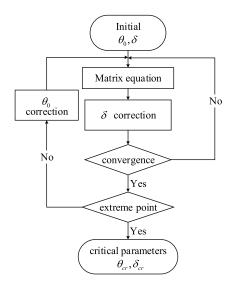
FIGURE 1. Flow chart for the indirect numerical method.
