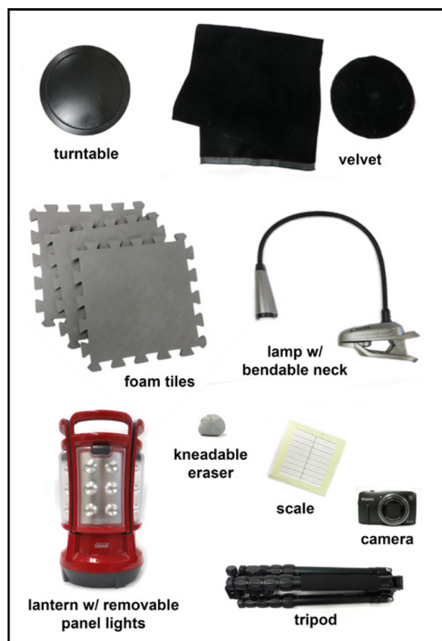
FIGURE 1. Materials used by the authors to create a portable photogrammetry rig.
