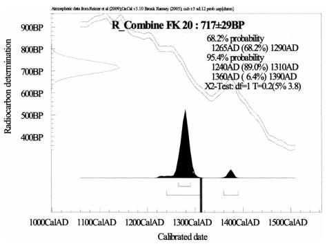
Figure 3 Timing for foundation of the Medieval monastery based on combined <sup>14</sup>C ages of the 1st and 2nd fractions of mortar, each collected for 3 s. The historical date is known to be after AD 1308 (vertical line), when King Albert I of Habsburg was murdered and the abbey was founded at the site.
