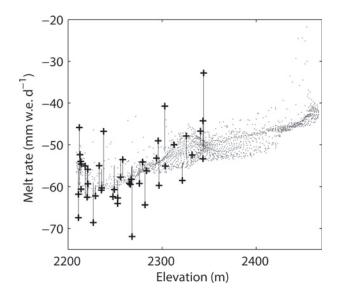
**Fig. 4.** Total surface melt from 6 July to 6 September 2009 computed using a melt model for all mesh gridpoints (·) and measured in the field at the stakes (+). The length of the vertical lines indicates the difference between the measured and computed melt at the stake locations.
