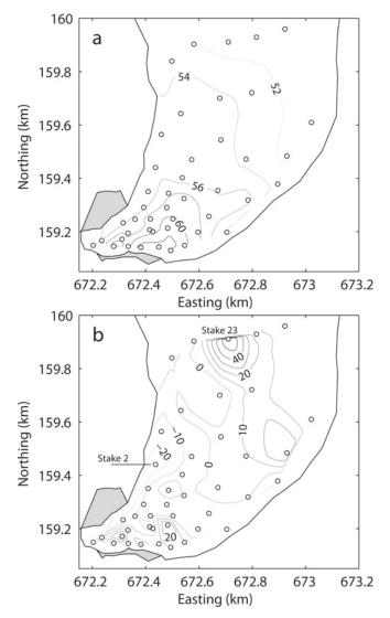
**Fig. 5.** (a) Melt rates (mm w.e.  $d^{-1}$ ) computed for the period 6 July to 6 September 2009; and (b) relative deviations from the observed values, ( $M_{\text{comp}}/M_{\text{meas}} - 1$ )× 100%. The locations of ablation stakes are indicated by circles.
