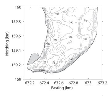
Fig. 8. Potential solar radiation computed for 29 July 2009 (W m<sup>-2</sup>). The contour intervals are 5 W m<sup>-2</sup>.
