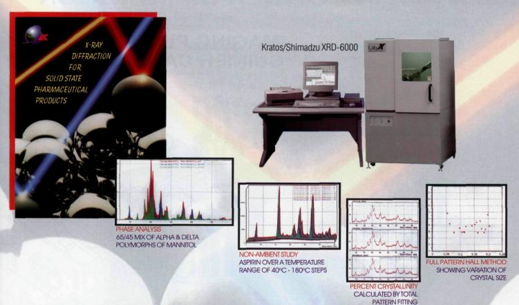
X-Ray Diffraction is a unique analytical tool for solid state pharmaceutical products to unambiguously characterize their solid state nature. Many parameters required by the FDA, legal patent issues and drug performance are only accessible by utilizing X-Ray Diffraction.
