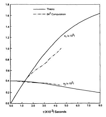
Figure 2. Amplitude variation as a function of time for a resonant pair of modes with the initial maximum isopycnal slope of the short wave equal to 0.42.
