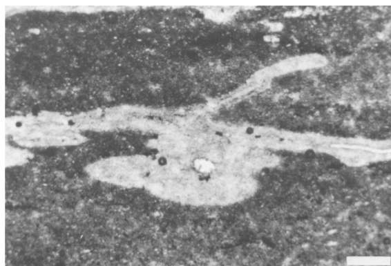
Figure 7. Photomicrograph of thin section of unweathered rock showing tracks and trails of a burrowing organism. Sample was collected from the upper yellow-brown shale (location 36G, Figure 1), Roger County, Oklahoma. The total organic carbon content is 0.4%. Plane polarized light. Bar scale = 250 \mu\text{m} .
