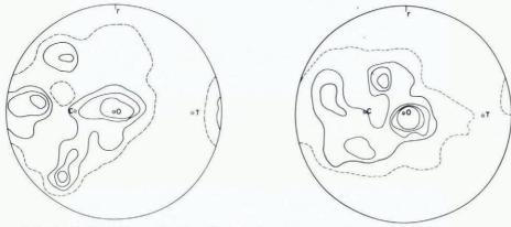
Fig. 8. c-axis fabrics of artificial ice samples after deformation in torsion-compression at -0.10°C. Symbols are defined in the caption to Figure 3.
