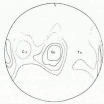
Fig. 5. c-axis fabric of specimen VB 50 after deformation in torsion. The contours are at densities of 1, 2, 4, and 6% in 1% of the area. Total strain: 24%; number of c-axes measured: 140. Symbols are defined in the caption to Figure 3.
