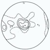
Fig. 3. c-axis fabric of specimen A2 after deformation in torsion. The contours are at densities of 2, 4, 6, and 8% in 1% of the area. C (compression), T (tension), and r are the axes of principal stresses. O is the axis of torsion. Total strain: 44%; number of c-axes measured: 106.
