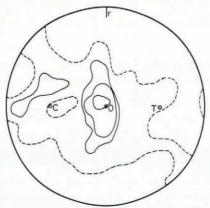
Fig. 6. c-axis of fabric specimen A3 after deformation in torsion. The contour are at densities of 0.5, 3, 5, and 10% in 1% of the area. Total strain: 45%; number of c-axes measured: 144. Symbols are defined in the caption to Figure 3.
