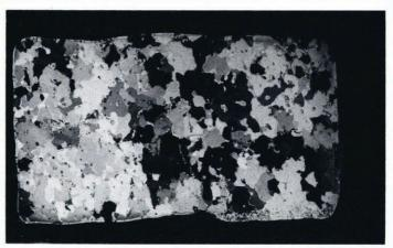
Fig. 10. Thin-section photograph of crystalline texture of ice specimen TC A4 between crossed polaroids after deformation in torsion-compression.  $\tau=2.8$  bar and  $\sigma=2.7$  bar; dimensions of the thin section:  $\theta$  cm $\times$  4.6 cm. The torsion axis was parallel to the direction containing the largest dimension of the thin-section. The radial direction was perpendicular to the thin section.
