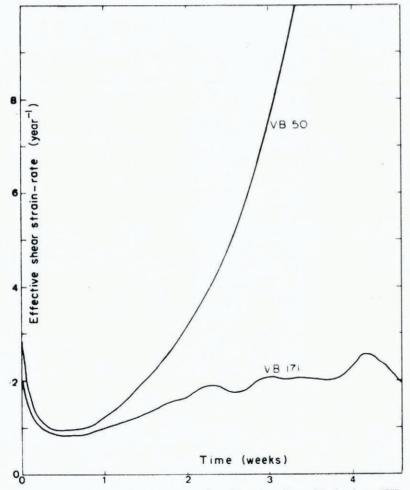
Fig. 4. Effective shear strain-rate versus time for a creep test performed in torsion. Natural ice samples:  $\tau$  (VB 50) = 3.0 bar;  $\tau$  (VB 171) = 2.7 bar; temperature  $T = -1.0^{\circ}$ C.
