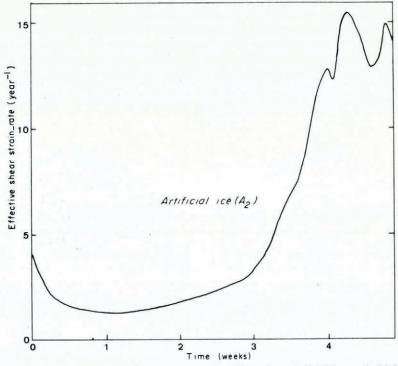
Fig. 2. Effective shear strain-rate versus time for a creep test performed in torsion. Artificial ice sample (A2).  $\tau = 2.50$  bar, temperature  $T = -1.0^{\circ}C$ .
