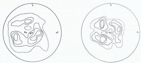
Fig. 7. c-axis fabrics of artificial ice samples after deformation in torsion-compression at -0.10°C. Symbols are defined in the caption to Figure 3.
