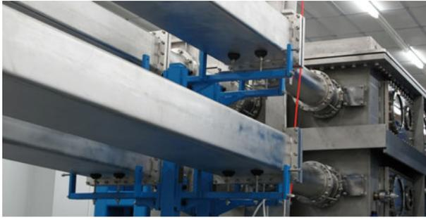
**Figure 10.** Beams bounded together preventing error accumulation.
