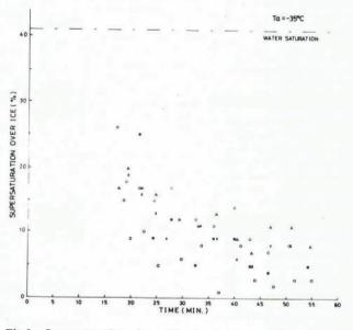
Fig.3. Supersaturation in cold chamber as a function of time.
