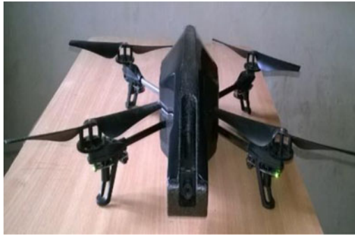
Figure 2. Parrot AR drone quadrotor version 2.0.
