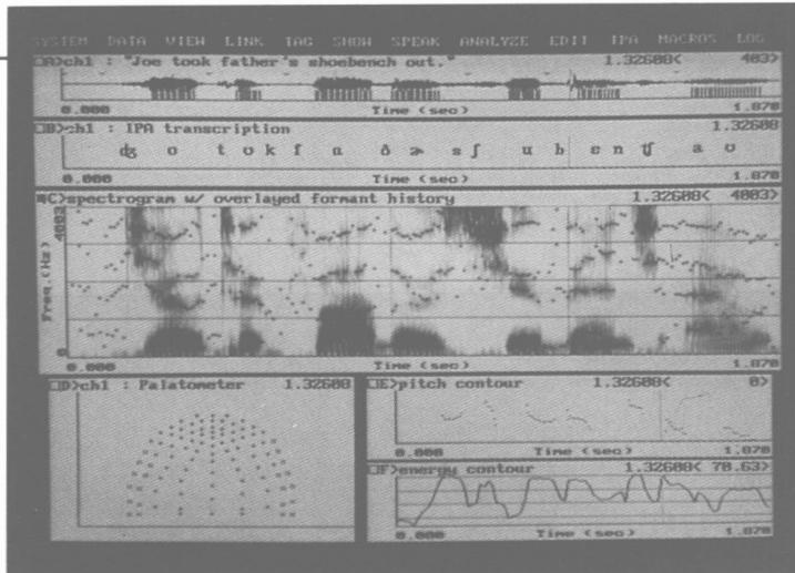
Multiple windows of analysis including speech waveform, phonetic transcription (time-linked to waveform), spectrogram overlaid with formant trace, pitch and energy contour and lingua-palatal contact in lower left is linked to cursor in spectrogram.
