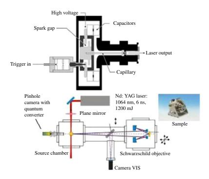
Figure 1. Experimental systems: scheme of the CDL system operated in Prague<sup>[15, 16]</sup> and scheme of the LPP system operated at LLG in Göttingen<sup>[17]</sup>.
