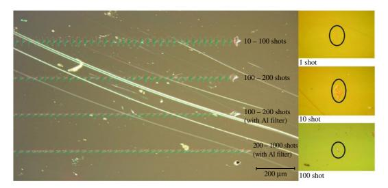
**Figure 3.** CDL at a wavelength of 46.9 nm: caustic measurement wavelength 46.9 nm (below) and ablation measurement (top). The shape of the crater is almost the same along the line of the caustic. Looking at the image on the right it can be seen that the annular form is preserved although, on increasing the number of shots, its dimensions increase.
