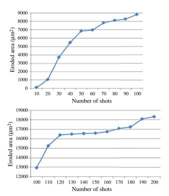
**Figure 4.** CDL at a wavelength of 46.9 nm: eroded area on number of shots (100–200 shots, bottom; 10–100 shots, top).
