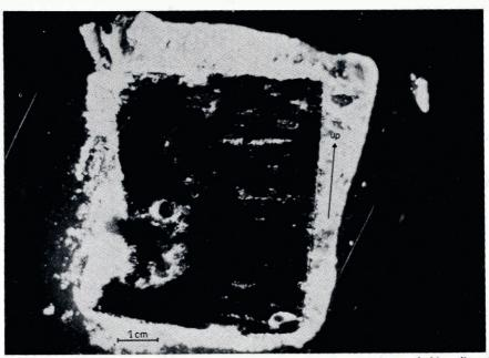
Fig. 2. Vertical thin section of waste-waler sludge ice taken from the "dirty ice" region and photographed in ordinary light. The section has its long side vertically oriented and clear ice around the edges of the section was used to freeze the section in position.
