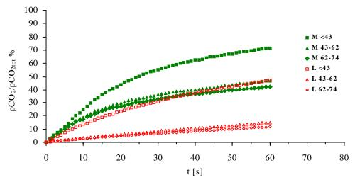
Figure 2 The dependence of the rate of reaction on grain size for a mortar (M) and a limestone (L). The grain size ranges were 62–74, 43–62 and <43 microns.
