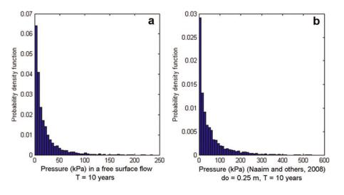
Fig. 13. Dynamic pressure in the free surface flow (a) versus impact pressure evaluated with Naaim's formula (b) for a decennial avalanche.
