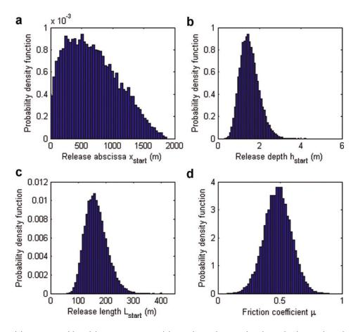
**Fig. 7.** Distribution of the input variables of the propagation model: (a) release abscissa, (b) release depth, (c) release length and (d) friction coefficient  $\mu$ . Parameters of the magnitude model equal their posterior mean  $\hat{\theta}_M$ . Release lengths are derived from release depths using Equation (10).
