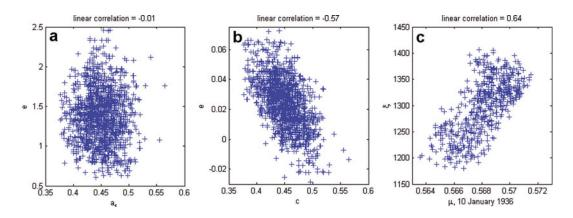
**Fig. 6.** Three joint posterior distributions. Three unknown pairs are presented: (a) two parameters with no correlation; (b) two parameters with a high negative correlation; and (c) the two highly positively correlated friction coefficients for the 10 January 1936 avalanche.
