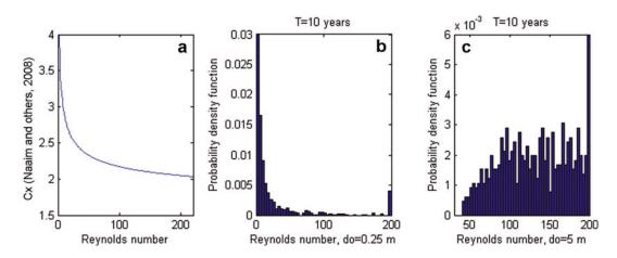
**Fig. 11.** Drag coefficient versus Reynolds number (a) and Reynolds number for a decennial avalanche for two sizes of obstacle, 0.25 m (b) and 5 m (c). The relationship between Reynolds number and drag coefficient is for a prismatic obstacle shape.
