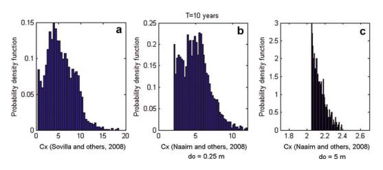
Fig. 12. Drag coefficient for a decennial avalanche, evaluated with Savilla's experimental formula (a) and Naaim's semi-empirical formula for two sizes of obstacle, 0.25 m (b) and 5 m (c).
