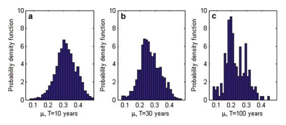
Fig. 9. Distribution of the Coulombian friction coefficient versus return periods of (a) 10 years, (b) 30 years and (c) 100 years. Only the exceedances of the corresponding abscissa are retained (e.g. for T = 30 years, the abscissa has a 0.033 annual probability of being reached).
