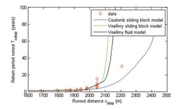
**Fig. 14.** Comparison with sliding block propagation models. The Voellmy fluid model of this paper is compared with the statistical–dynamical sliding block model with a Coulombian friction law from Eckert and others (2007b) and with a statistical–dynamical sliding block model with a Voellmy friction law.
