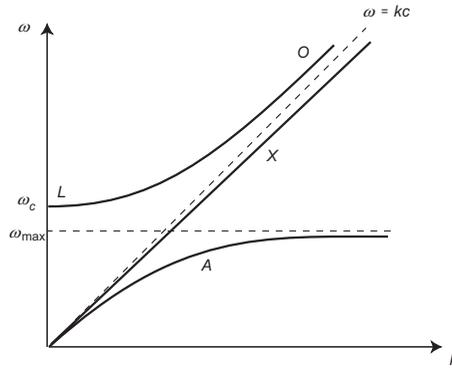
**Figure 1.** Dispersion curves for a pulsar plasma well below the cyclotron resonance: the cutoff is in the L-O mode, and the resonance is in the Alfvén (A) mode. Not shown is a small region near  $\omega_c \gamma$  for nearly parallel propagation, where the O-mode dispersion curve crosses the light line (shown dashed), cf. (Melrose *et al.* 1999).
