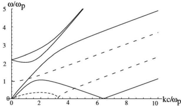
**Figure 2.** Dispersion curves  $\omega$  vs  $k$  in normalized units for parallel propagation in a cold counter-streaming plasma with  $\beta = 0.3$ ,  $\Omega_e = 2\omega_p$ . Dotted lines show imaginary parts, dashed lines show longitudinal real parts and solid lines show transverse real parts (Verdon & Melrose 2008).
