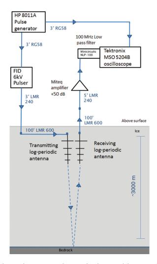
**Fig. 1.** The experimental set-up for the ground bounce with low-frequency antennas. We used an FID Technologies 6 kV high-voltage pulser (http://www.fidtechnologies.com), triggered by a Hewlett Packard 8011A pulse generator to transmit through a log-periodic antenna. We used a second log-periodic antenna coupled to a +50 dB Miteq amplifier to boost the received signal and a Tektronix MSO5204B to record the data.
