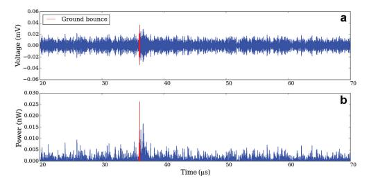
**Fig. 3.** (a) The received voltage in a 50  $\Omega$  receiver as a function of time with the log-periodic antennas buried in the snow, pointed downward. A large reflection is evident at 36.1 µs (highlighted in red), consistent with a depth of  $3014^{+48}_{-50}$  m. (b) The power received as a function of time, derived from the top panel. The red region denotes the 200 ns wide time window used for analysis.
