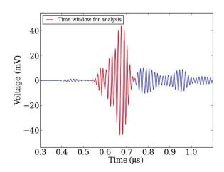
**Fig. 5.** The transmitted impulsive signal received directly through 46 m of air, Butterworth filtered to 65–85 MHz. The system used is the same as for the ground bounce, but with 40 dB of additional attenuation on the receiver. The red region shows the time window used for analysis (200 ns wide).
