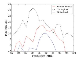
**Fig. 4.** The power spectral density of the received ground bounce signal compared to the noise level in the trace. For comparison, the power spectral density of the through-air normalization signal, with 40 dB of additional attenuation compared to the ground bounce signal, is shown with a dashed line. All data have been filtered (65–85 MHz), time-windowed and zero-padded in the same way.
