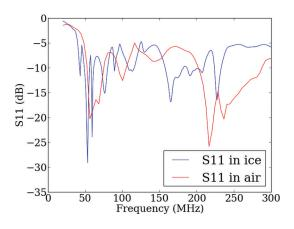
**Fig. 2.** The return  $loss (S_{11})$  of the log-periodic antenna used for the ground bounce measurement for the antenna buried below the surface and packed with snow (blue), compared to the same antenna in air (red).
