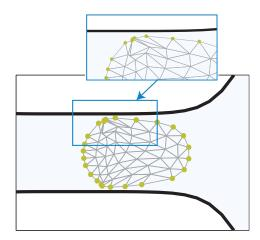
FIGURE 10. Mesh distortion due to motion with large deformations. Since in the limit of small relaxation timescale, the constitutive law for viscoelasticity describes a viscous fluid, the method does not guarantee to preserve the mesh spacing as the material deforms. Thus, for large deformations, in the case of moving, deforming structure, re-meshing algorithms need to be considered.
