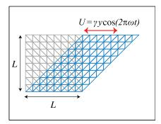
FIGURE 2. Schematic for the oscillatory linear shear test. A square viscoelastic material undergoes a prescribed oscillatory motion in the horizontal direction as given by equation (3.2) with amplitude  $\gamma$  and frequency  $\omega$ . The initial material configuration is shown in grey while the later in time configuration is in blue (online). We note that the deformation is not drawn to scale.
