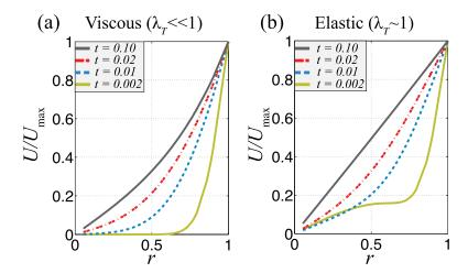
FIGURE 7. Velocity profiles across the radially symmetric material for different relaxation timescales. Shown here are different time plots of the scaled radial velocity  $U_r(r,t)$  by the maximum velocity  $U_{\rm max} = 1.0 \times 10^{-2}$ . The time-space evolution of the scaled radial velocity is illustrated for the case of (a) small relaxation timescale,  $\lambda_T = 0.05$ , and (b) relaxation timescale much longer than observable time,  $\lambda_T = 2$ .
