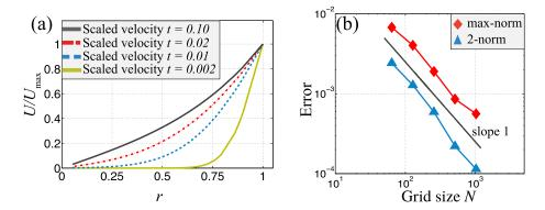
FIGURE 6. Relative error in the velocity profile of the immersed structure for a linear expansion test. (a) Given here is the velocity  $U_r(r,t)$  in the radial direction at several time points divided by the maximum velocity  $U_{\text{max}} = 1.0 \times 10^{-2}$ . (b) The 2-norm and max-norm of the difference between the truncated series solution of the velocity field and numerical solution scaled by the maximum velocity at t = 0.1 is plotted for different grid sizes.
