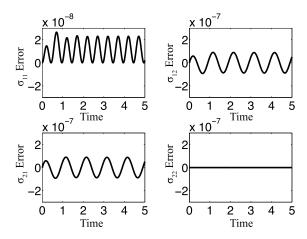
FIGURE 4. Comparison of a full 2D prescribed motion simulation with linear viscoelasticity for a small amplitude oscillatory shear test. Shown here are the relative differences in the stress components between the analytically computed stress for linearized Maxwell model and the computed stress in the prescribed motion simulation; both stress measurements are normalized by the maximum stress over time.
