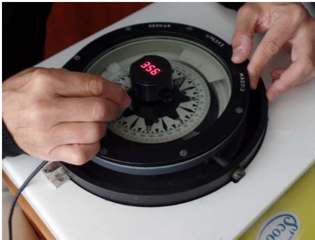
Figure 4. Ship's magnetic compass while adjusting the IMC sensor.
