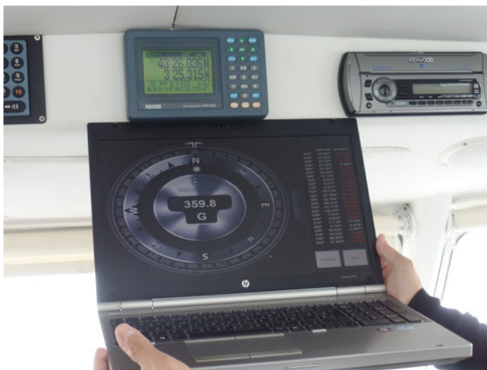
Figure 8. True course and COG comparison. True course from the satellite compass is shown on the IMC.
