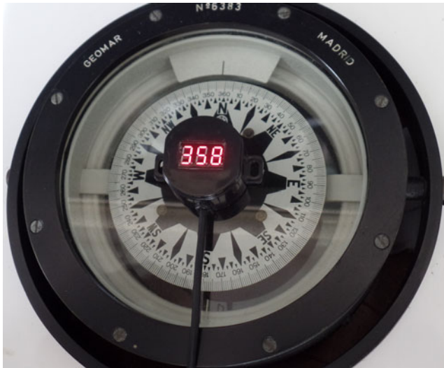
Figure 5. Ship's magnetic compass with the IMC sensor already adjusted.
