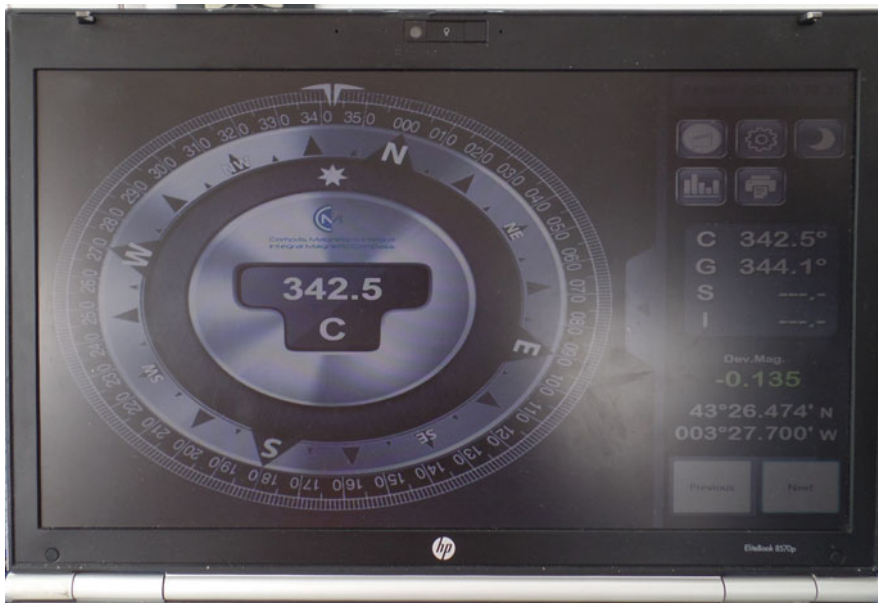
Figure 6. IMC with the compass course, true course obtained from the satellite compass, position obtained from GPS and magnetic declination obtained from the NOAA calculator.
