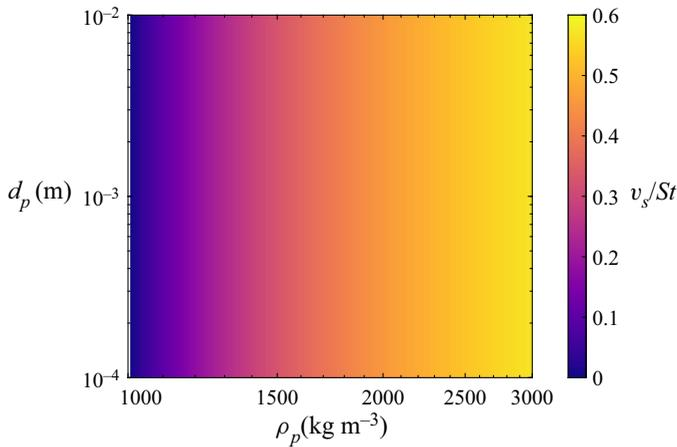
Figure 13. Ratio of dimensionless terminal velocity to Stokes number for deep-water waves calculated with the Schiller–Naumann drag model for  $\rho = 10^3 \text{ kg m}^{-3}$  and  $\nu = 10^{-6} \text{ m}^2 \text{ s}^{-1}$ .
