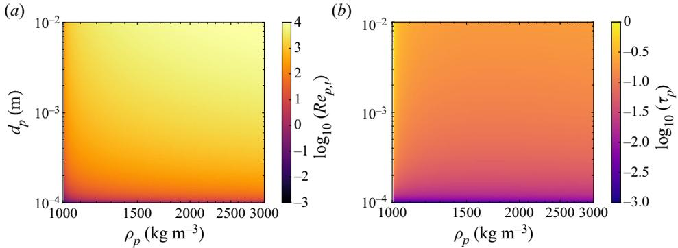
Figure 1. Particle parameters calculated with the Schiller–Naumann drag model for  $\rho = 10^3 \text{ kg m}^{-3}$  and  $\nu = 10^{-6} \text{ m}^2 \text{ s}^{-1}$ : (a) particle Reynolds number at terminal velocity; (b) particle time scale in seconds.
