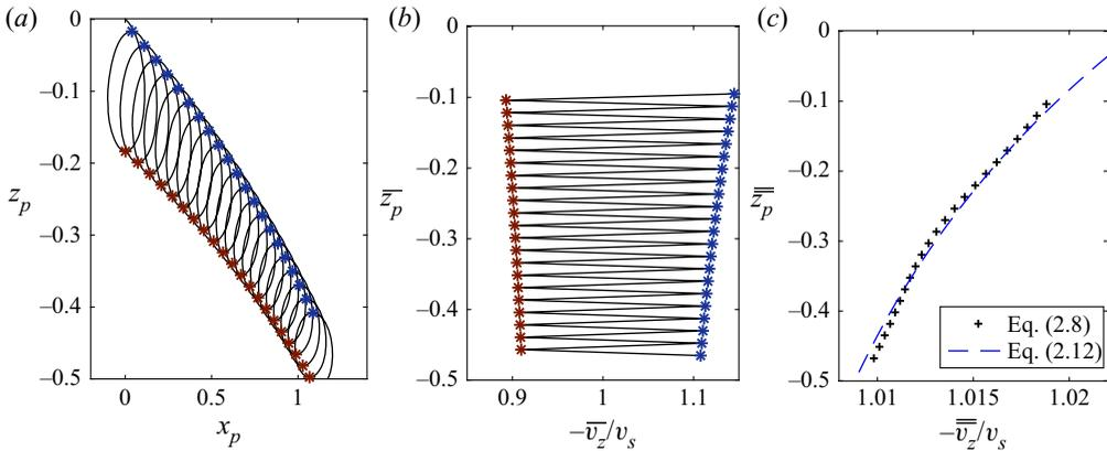
Figure 11. Particle trajectory and wave-averaged drifts for  $kh = 1$ ,  $ka = 0.1$ ,  $\gamma = 1.05$ ,  $St_{SN,t} = 0.065$ ,  $Re_{p,t} = 6.5$ . (a) Particle trajectories computed with the nonlinear drag model using the full dynamical equation for particle motion (2.8) with constant phase points marked with \*. (b) Wave-averaged vertical velocity with starting phase points marked. (c) Twice wave-averaged vertical velocity of the trajectory  $-\overline{\overline{v_z}}/v_s$ .
