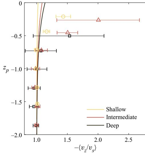
Figure 12. Experimental data (symbols) from Clark *et al.* (2020) compared with predicted vertical drift (2.12b) (solid lines). Different colours represent different experimental cases: ‘shallow’:  $ka = 0.15$ ,  $kh = 1.77$ ; ‘intermediate’:  $ka = 0.30$ ,  $kh = 3.8$ ; ‘deep’:  $ka = 0.37$ ,  $kh = 6.7$ . Error bars denote 95 % confidence intervals which were found by bootstrapping the experimental data.
