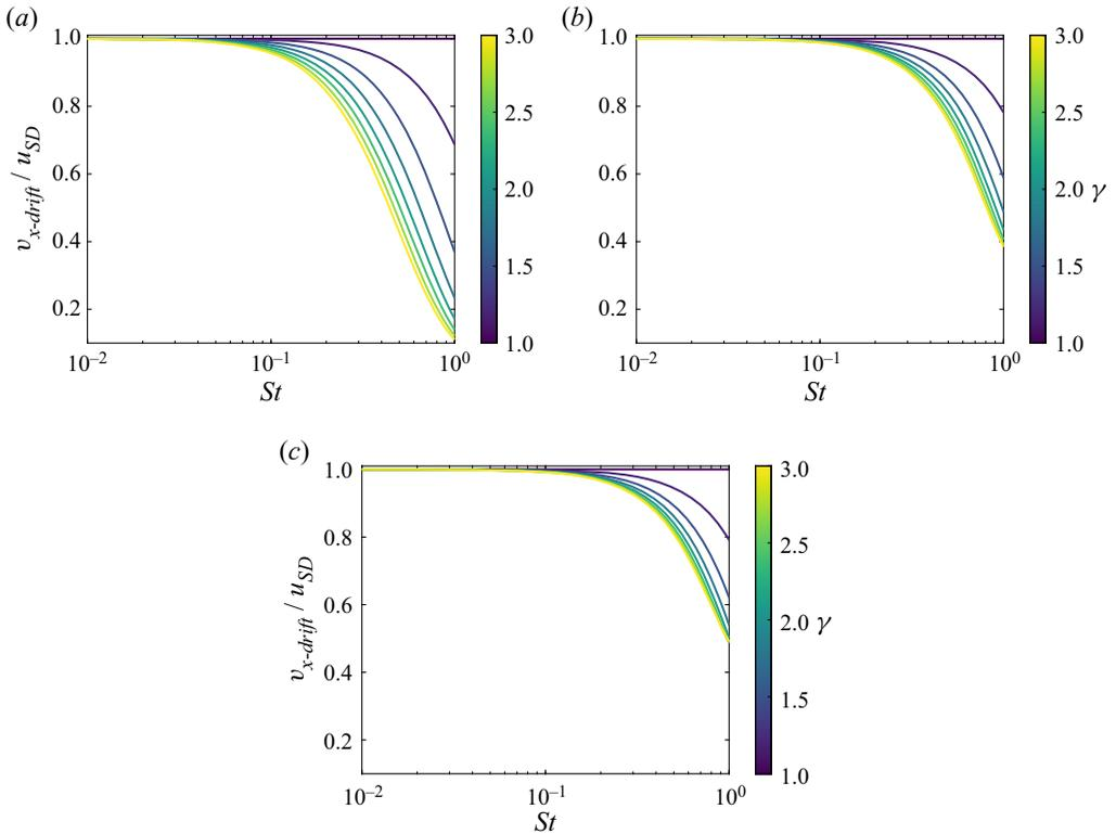
Figure 3. Horizontal drift for settling particles relative to tracer particles as functions of Stokes number  $St$  for different density ratios  $\gamma$  at different relative depths  $kh$ , calculated using (2.12a). Lines correspond to different density ratios,  $\gamma = 1, 1.2, 1.5, 1.8, 2.1, 2.4, 2.7, 3$ ; (a)  $kh = 0.3$ , (b)  $kh = 1.0$ , (c)  $kh = 3.0$ .
