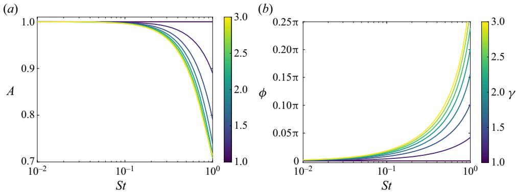
Figure 2. Particle motion parameters as functions of Stokes number  $St$  for different density ratios  $\gamma$  calculated using (2.11). (a) Amplitude  $A$  and (b) phase shift  $\phi$  of particle velocity relative to tracer particles. Lines correspond to a different density ratios,  $\gamma = 1, 1.2, 1.5, 1.8, 2.1, 2.4, 2.7, 3$ .
