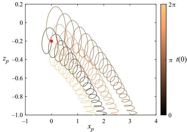
Figure 6. Particle trajectories computed with the linear drag model using (2.10) for particles released continuously at  $(x, z) = (0, -0.2)$  (red asterisk) for  $ka = 0.2$ ,  $kh = 1$ ,  $\gamma = 1.1$  and  $St = 0.1$ . Trajectories are coloured according to their initial starting time.
