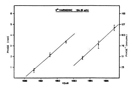
Figure 2. Phase variation of the ninth harmonic of a day over the period 1980-1985. The phases are obtained for each annual series by means of a sine wave fitting procedure; the six annual series have the same time reference:  $1^{SL}$  April 1980 at  $0^{h}$  G.M.T.
