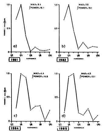
Figure 1. Daily harmonics power profile corresponding to the four yearly considered series. Each point represents the power under a particular harmonic; the integrated power for all of them and its maximum individual value are shown, in (m/s)\*\*2/ $\mu$ Hz.
