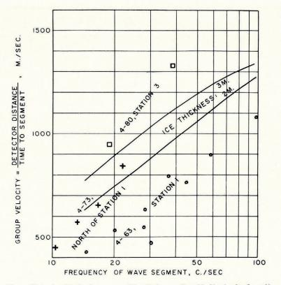
Fig. 5. Dispersion data for flexure waves (theoretical curves from Hunkins (1960, fig. 13))
