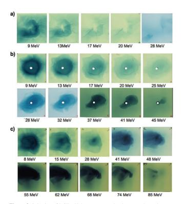
**Figure 8.** Selection of RCF which were exposed to laser-accelerated proton beams. The energy of protons which are fully stopped in the particular foil are written underneath each layer. Shown are examples for: (a) a shot with a ns-prepulse with a contrast ratio around  $10^6$ , (b) a shot after removing the prepulse and (c) a shot using the full aberration control.
