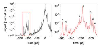
**Figure 4.** Temporal profile of the PHELIX pulse in 2012 using the uOPA with a gain of  $10^4$ . The pulse was measured with a third order cross-correlator (Sequoia, Amplitude Technologies). The right graph shows an enlargement of the red framed region of the left graph.
