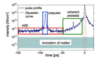
**Figure 1.** Temporal profile of the PHELIX pulse in 2010 before the application of pulse cleaning techniques, measured with a third order cross-correlator (Sequoia, Amplitude Technologies). The curve has been scaled to a peak intensity of  $10^{20}$  W cm<sup>-2</sup>. The shaded area illustrates the ionization threshold for typical target materials. The red dashed line shows a Gaussian function with the same FWHM as the pulse (blue).
