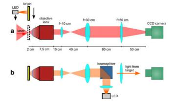
**Figure 6.** Schematical setup of the focus and target alignment system. (a) The laser focus is imaged on the camera while the target is moved to the side. A transparent target is mapped on the camera by transmitting the light from the LED inside the target chamber through the target. (b) For alignment of opaque targets the LED light is coupled into the diagnostics beamline using a beamsplitter cube and light coming back from the target is imaged onto the camera.
